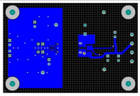
Figure 10-3. Bottom-Layer Traces and Copper (Flipped)
