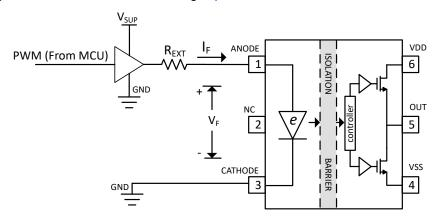
Figure 8-2. Driving the Input Stage of UCC23525 with One Buffer and Anode Resistor
