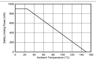
Figure 5-2. Thermal Derating Curve for Safety **Limiting Power**
