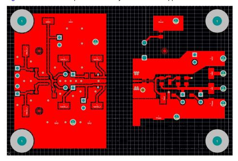
Figure 10-2. Top-Layer Traces and Copper
