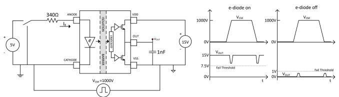
Figure 6-3. CMTI Test Circuit for UCC23525
