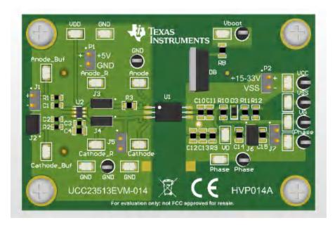
Figure 10-4. 3-D PCB View
