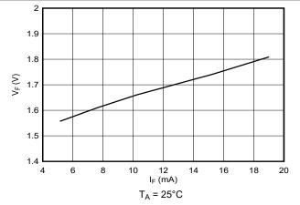
Figure 5-6. Forward voltage drop versus Forward current
