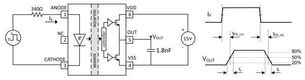
Figure 6-1.  $I_F$  to  $V_{OUT}$  Propagation Delay, Rise Time and Fall Time
