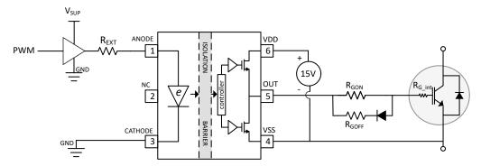
Figure 8-1. Typical Application Circuit for UCC23525 to Drive IGBT
