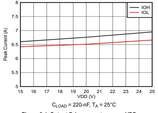
Figure 5-4. Output Drive currents versus VDD
