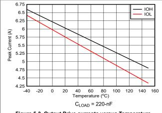
Figure 5-3. Output Drive currents versus Temperature
