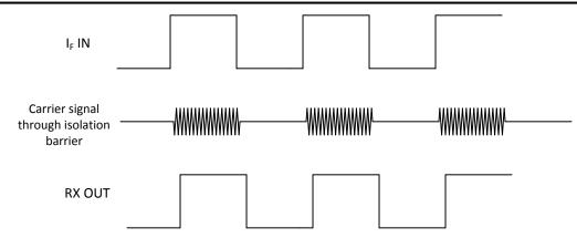
Figure 7-2. On-Off Keying (OOK) Based Modulation Scheme
